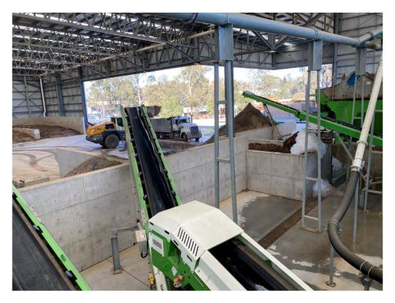
Plate 6 - Sand, organics and recovered aggregate conveyor belts
