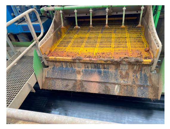
Plate 3 – Aggregate sprayers
