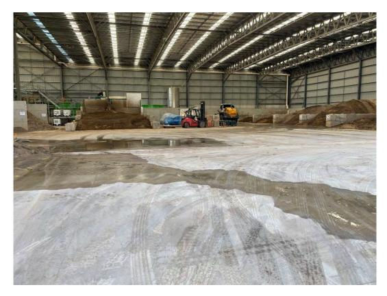
Plate 11 – Clean workshop floor showing appropriately bunded storage areas for stockpiles
